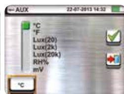
Selection of measurement type with external probe
