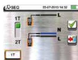
Selection of measurement type of phase sequence
