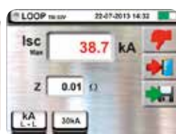
Negative result of breaking capacity test
