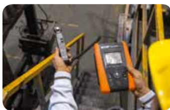
Lux measurement with accessory HT53/05.
