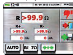
Continuity of protective conductors: Measurement result negative
