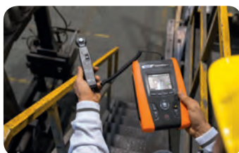
Lux measurement with accessory HT53/05.
