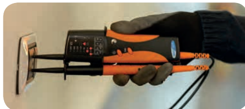
Multimeter function with display and LED indication.
